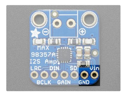
This is the power for the amplifier and logic of the amplifier. You can provide 2.5V up to 5.5V. Note that at 5V you can end up putting up to 2.8W into your speaker, so make sure your power supply can easily handle up to 650mA and we recommend a power supply spec'd for at least 800mA to give yourself some 'room'
