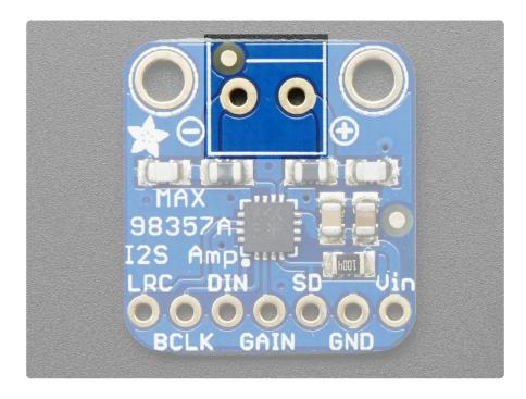
This amplifier is designed to drive moving coil loudpeakers only. Speaker impedence must be  $4\Omega$  or more. The output signal is a 330KHz PWM square wave with a duty cycle proportional to the audio signal. The inductance of the speaker coil serves as a low-pass filter to average out the high-frequency components. Do not try to use this as a pre-amplifier.
